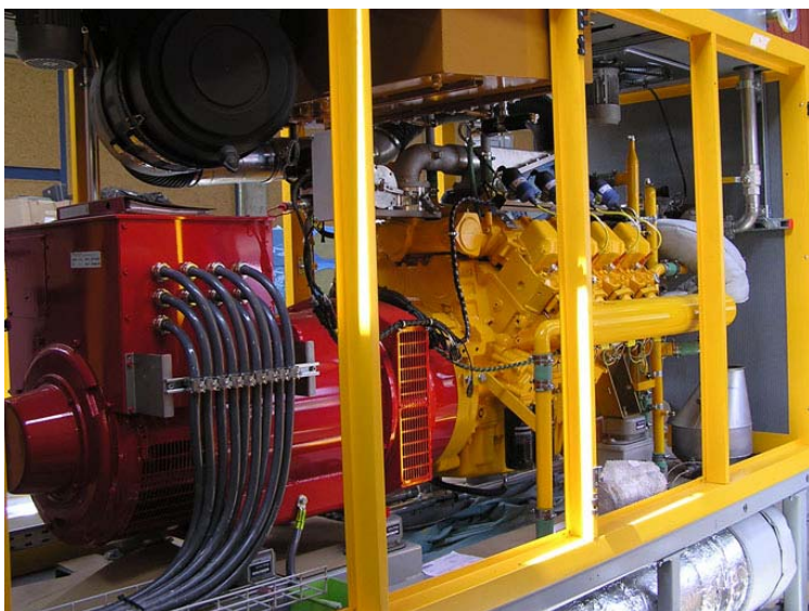
Figure 8-5 Cogeneration unit with a 8-cylinder “Swissmotor”. Electric efficiency 38%, electricity generation 280 kW, heating capacity 389 kW, \text{NO}_x < 50 \text{ mg/Nm}^3 [Avesco, CH-4901 Langenthal]
